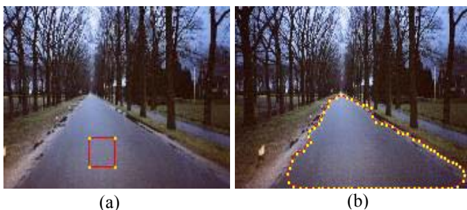
Figure 1: Active contour model and balloon. (a). Initial curve. (b). The lane is detected.
